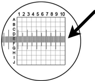
Line up one of the larger lines on the stage micrometer with the right edge of the reticle grid. Measure the distance across the row of 10 squares. Enter this distance as “Width 1” on the Scaling Factor worksheet.
