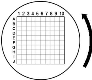
After the reticle installation, rotate the eyepiece until the grid labels are right side up and legible.
