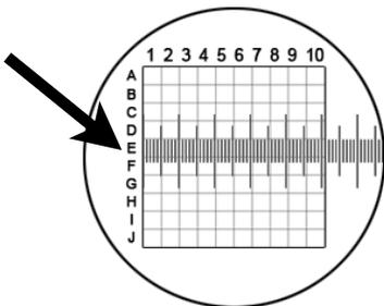
Line up one of the larger lines on the stage micrometer with the left edge of the reticle grid and measure the entire grid again. Enter this as “Width 2” on the Scaling Factor worksheet.
